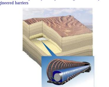
Figure 45 Yucca Mountain repository concept, showing the tunnel layout design and engineered barriers
