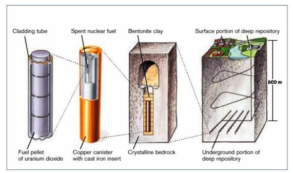
Multiple barriers prevent the radionuclides from reaching the ground surface. Source: Guais (2003).
