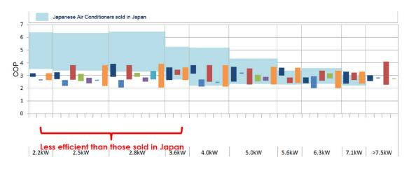
Figure 7-3: Comparative Efficiencies of AC Models in Brunei Darussalam
