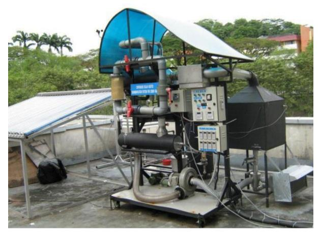
Figure 6-9: Solar dryer with chemical heat pump (for lemongrass)
