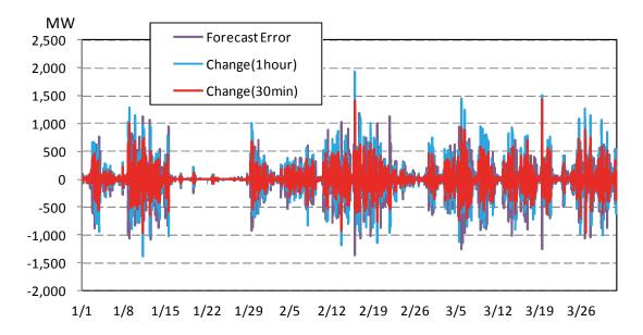
**Figure 4-11 Forecast Errors of Output of Wind Generation and Output Changes by Unit Time** Source: Bonneville Power Administration
