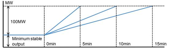
Figure 4-12 Concept Regarding Minimum Capacity Required to Increase Output by 100MW
