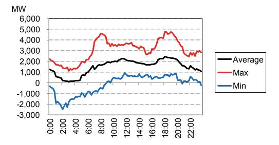
Figure 4-9 Distribution of Forecast Errors of Load
