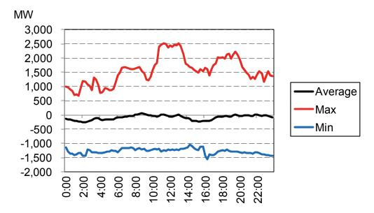
Figure 4-10 Distribution of Forecast Errors of Output of Wind Generation
