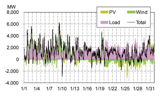
**Figure 4-8 Forecast Errors of Load, Output of Wind Generation and Output of PV Generation** Source: 50 Hertz Transmission
