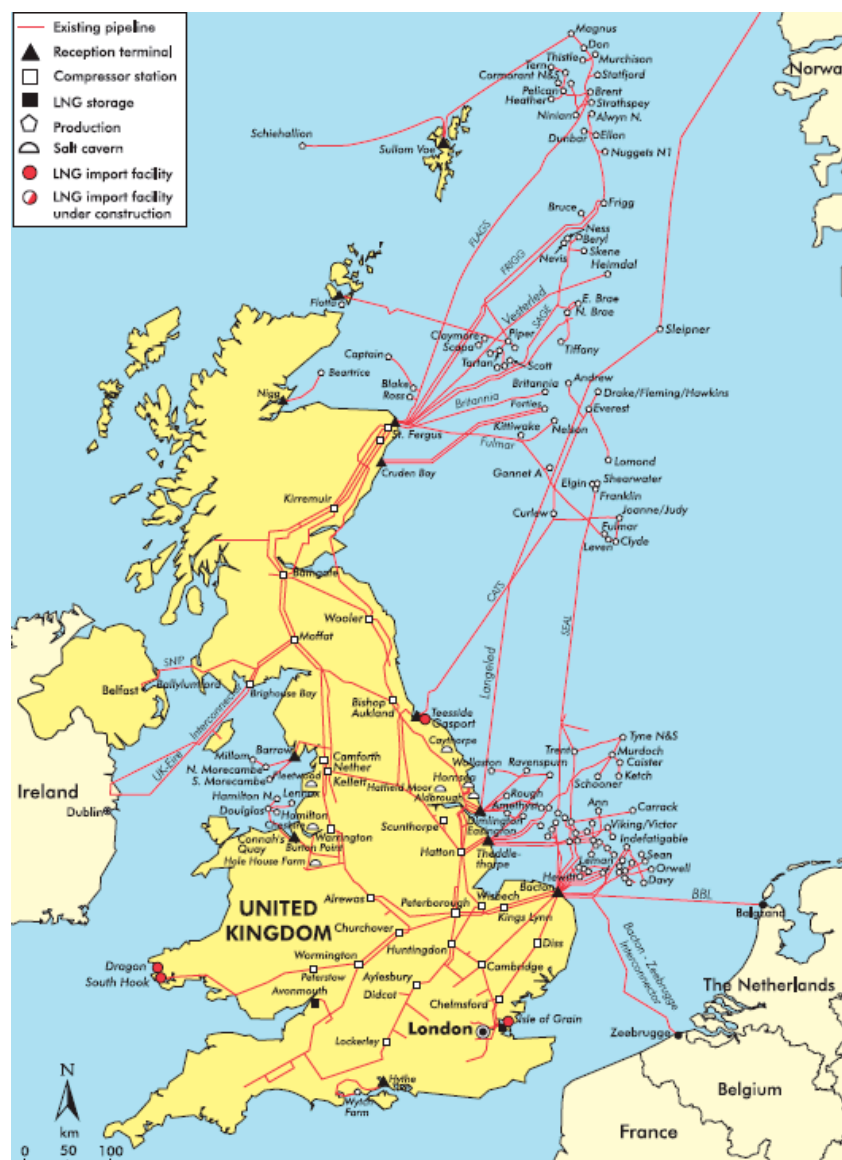
Figure 6.4 • Natural gas infrastructures in the UK
