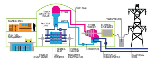
Figure 4 CANDU nuclear power reactor schematic diagram
