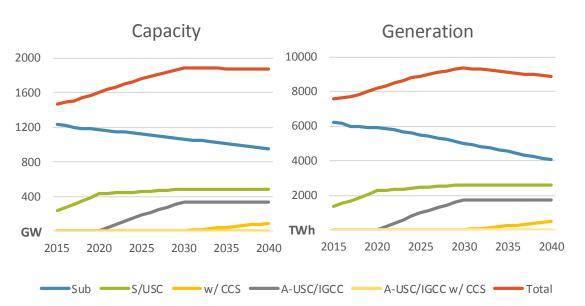
Figure 1.11: High coal scenario capacity and generation by technology type, APEC
