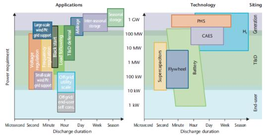
FIGURE 3-3. ELECTRICITY STORAGE APPLICATIONS AND TECHNOLOGIES
