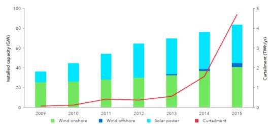
FIGURE 3-2. INSTALLED CAPACITY OF WIND AND SOLAR POWER AND CURTAILMENT IN GERMANY
