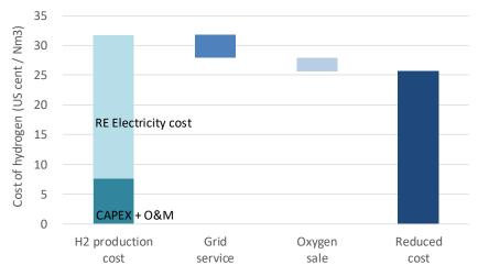
FIGURE 3-10. HYDROGEN PRODUCTION REDUCTION EFFECT BY DIVERSIFICATION OF REVENUE
