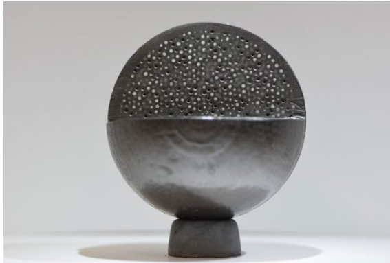
TRISO Fuel Pebble Cutaway
