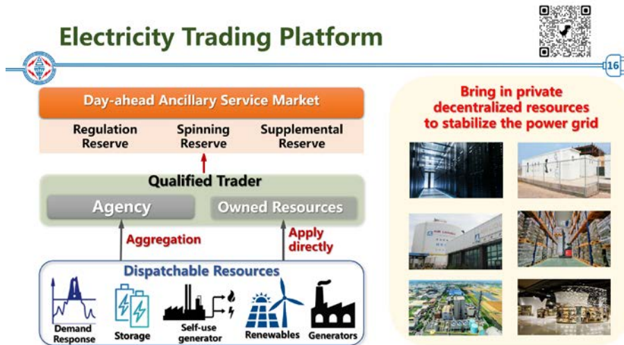
Figure 11 Structure of Taipower's Electricity Trading Platform
